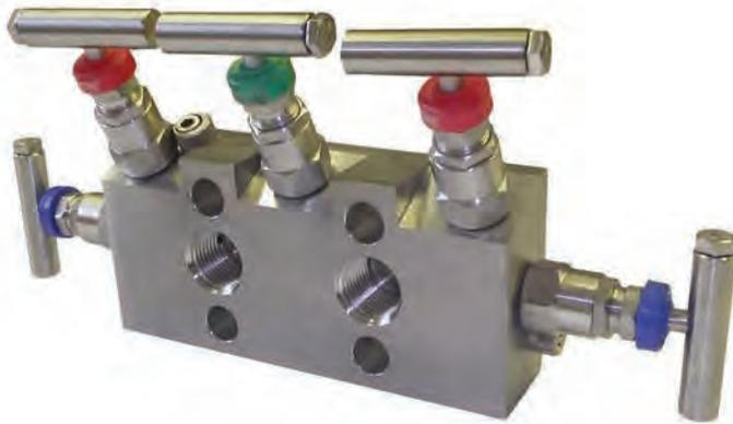
Direct style block mounted 5 valve manifold, instrument mount to pipe connection. Offering two isolation valves, two vent valves and one equalising valve (see attached drawing).
