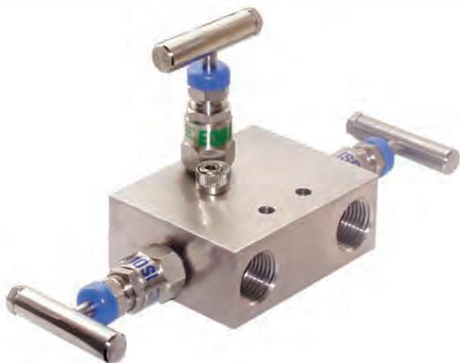
The three-valve isolation manifold remote mounted (pipe to pipe). Used mainly in differential pressure transmitters and static instrument applications. The '3VR' has two process isolation valves and one equalisation valve to equalise the two sides.
