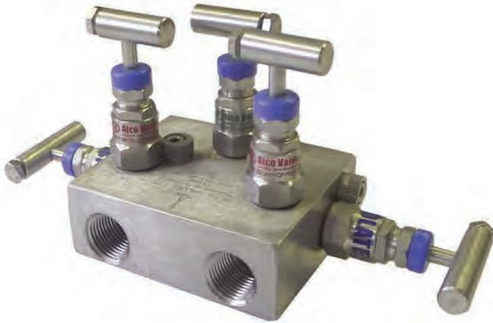
Remote mounted, pipe to pipe configuration five valve manifold. Offering two isolation valves, two vent valves and one equalising valve (see attached drawing). Used in differential pressure transmitters and static instrument applications.
