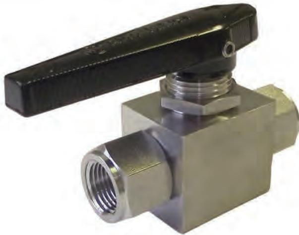
The single nut mounted ball valve is rated from vacuum up to 6,000psi. The single nut allows fast panel mounting. Max panel thickness is 11mm (dependant on valve size).
