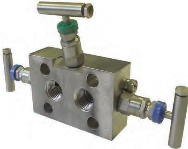
Direct mounted 3 valve manifold, instrument mount to pipe connection. Offering two isolation valves, and one equalising valve for differential pressure transmitter or static instrument applications. Unique bonnet locking cam for extra safety and for ease of maintenance
