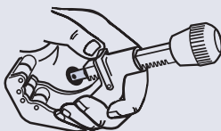
RATCHET FEED Ratchet release opens cutter instantly to maximum size.
