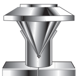
3 rollers in flaring cone. Flare formed above die block.
